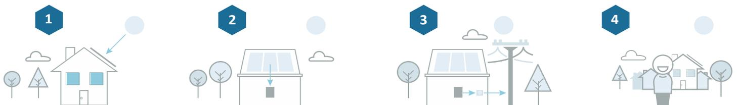
**PHOTOVOLTAIC EFFECT** - The phenomenon that occurs when photons, the "particles" in a beam of light, knock electrons loose from the atoms they strike. When this property of light is combined with the properties of semiconductors, electrons flow in one direction across a junction, setting up a voltage. With the addition of circuitry, current will flow and electric power will be available.
